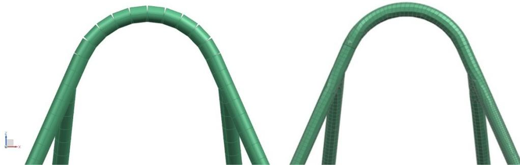
FIGURE 7. Main roll hoop curvature modeled by 1D beam elements (left) and 2D shell elements (right).
